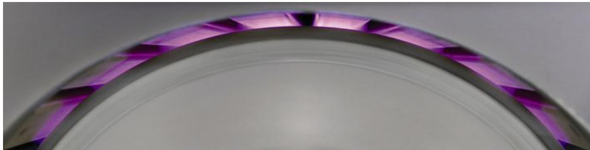
„Corona-Light“ in the discharge gap 8 ceramic electrodes / roller with ceramic coating
